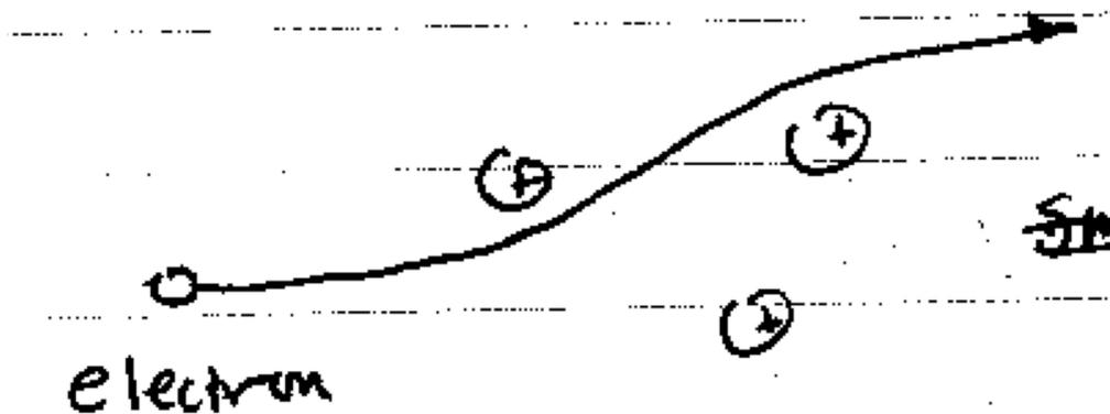
As charged particles (usually electrons) slow down in matter they are accelerated both longitudinally and transversely.
