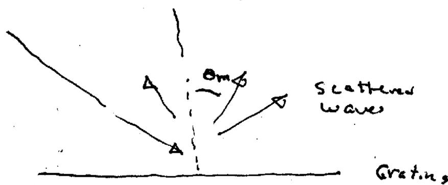
$$\frac{\omega}{c} \cos \theta_m = \sqrt{\frac{\omega^2}{c^2} - \left( \frac{\omega}{c} \sin \theta_i + m k_0 \right)^2}$$
