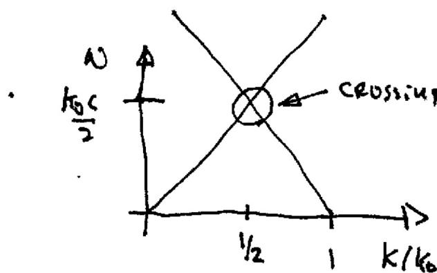
$$\left[ \frac{k_0 c \delta \omega}{c^2} - k_0 \delta k \right] \left[ \frac{k_0 c \delta \omega}{c^2} + k_0 \delta k \right] = \frac{\delta^2}{z^2} \left( \frac{k_0 \epsilon}{c^2} \right)^4$$
