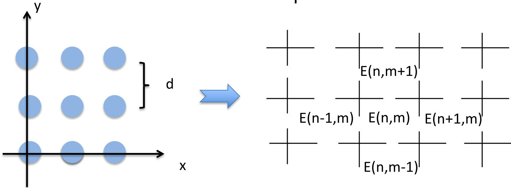
$$[\omega^2 - \omega_c^2]E(n,m) = \frac{\delta}{2}\omega_c^2 [E(n+1,m) + E(n-1,m) + E(n,m+1) + E(n,m-1)]$$
