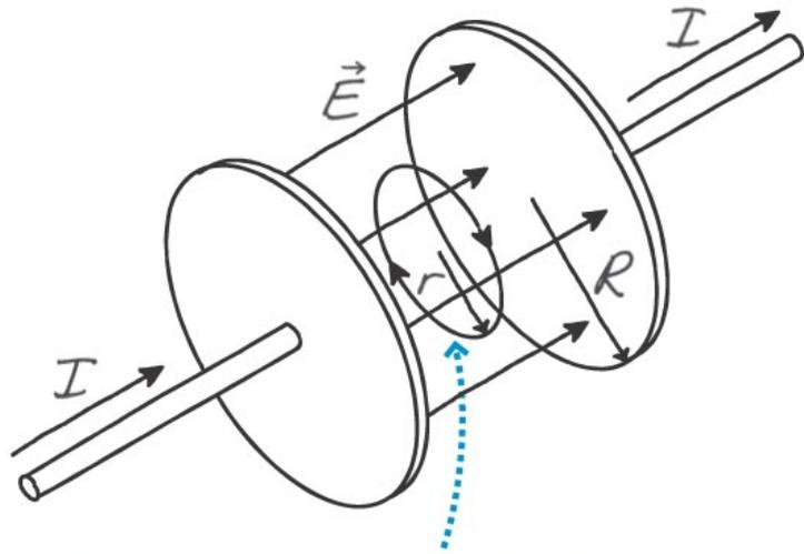
The magnetic field line is a circle concentric with the capacitor. The electric flux through this circle is  $\pi r^2 E$ .
