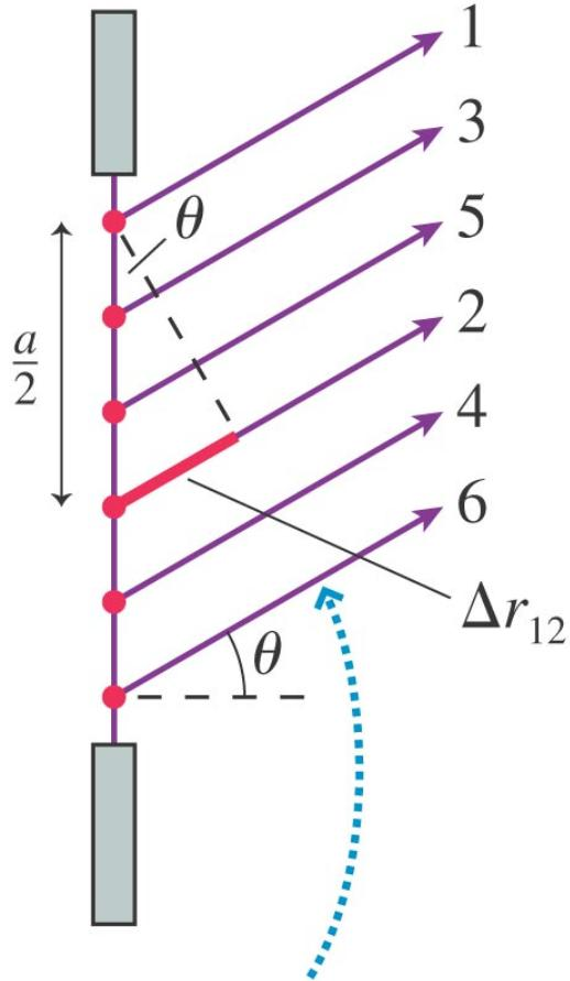
These wavelets all meet on the screen at angle  $\theta$ . Wavelet 2 travels distance  $\Delta r_{12} = (a/2) \sin \theta$  farther than wavelet 1.
