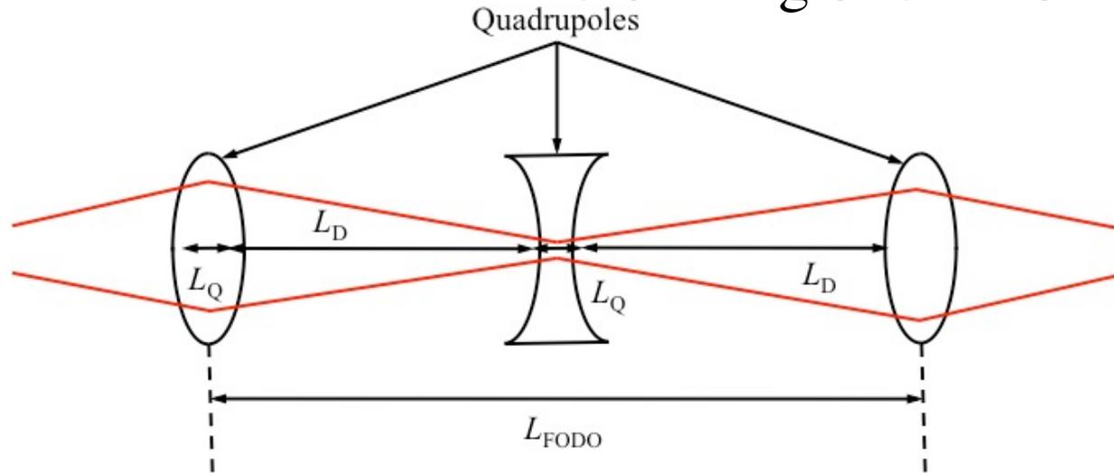
Qualitative explanation: beam passes through focusing quad when it is big (strong fields). Passes through defocusing quad when it is small (weak
