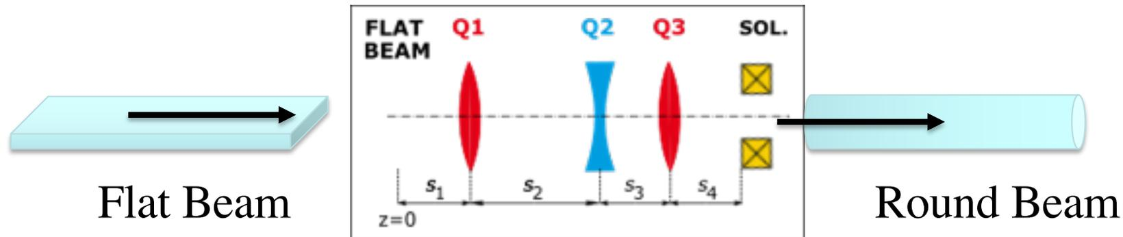
Flat to Round and Round to Flat transformers are proposed for cooling of hadron beams. Ya. Derbenev, Adapting optics for high-energy electron cooling, Tech. Rep. UM-HE-98-04-A (1998).
