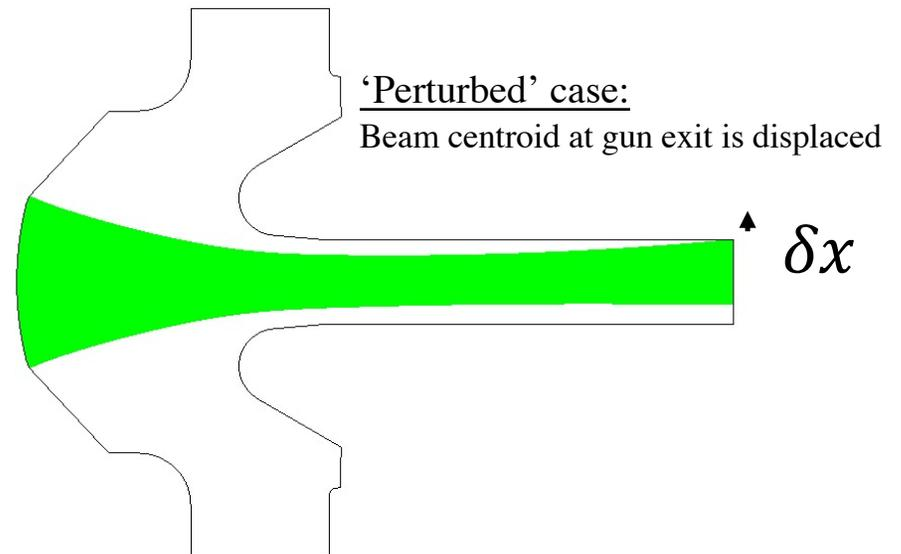
The adjoint method gives us a way to compute the displacement of the beam *without* re-running MICHELLE:
