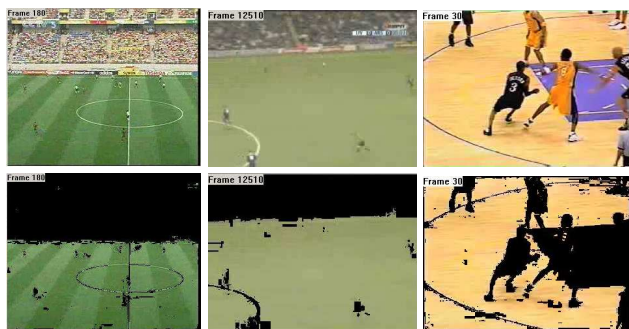
Fig. 1. Results for extracting the playground color. Top row: original frame; Bottom row: playground color pixels. From left to right: results for World Cup video A1, results for English Premier League video B2, results for NBA video D1.
