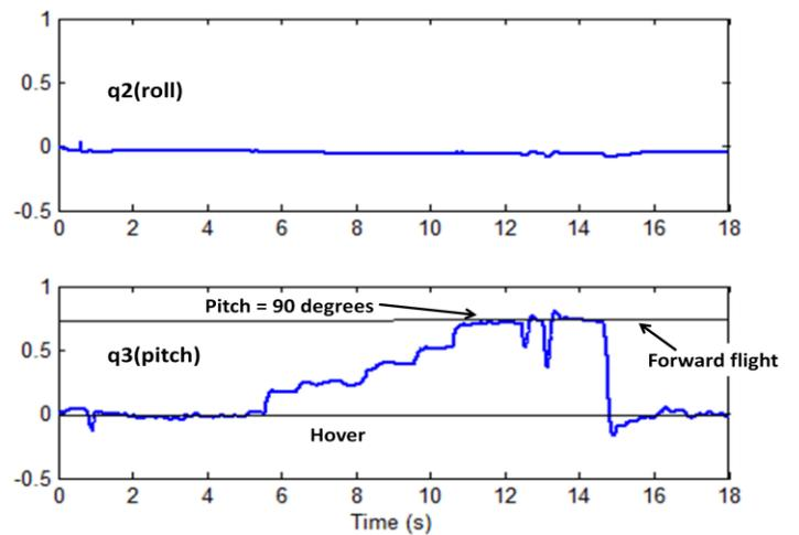
**Fig. 7. Bench top results of demonstrator undergoing change in desired quaternion,  $q_3$  with disturbances**
