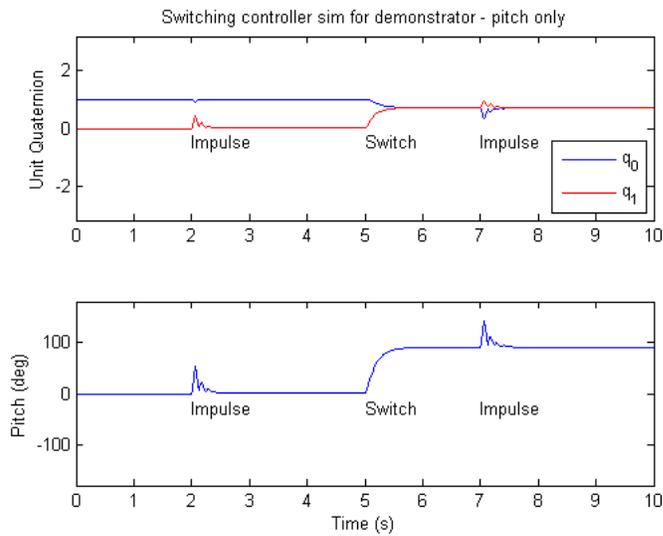
**Fig. 5: Simulation results of demonstrator undergoing change in desired quaternion with disturbances.**
