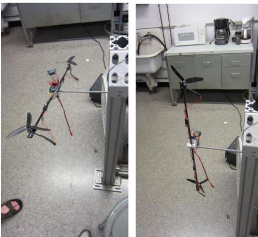
**Fig. 6. Bench top demonstrator, free to rotate in pitch**
