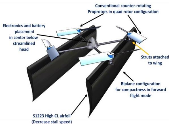
Fig. 1. Quad-rotor Biplane conceptual design
