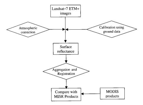
Figure 1. Flowchart of the validation process.
