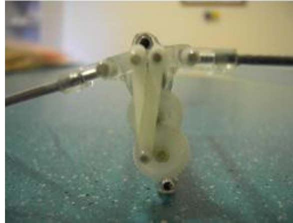
Figure 19: Chung Hua University MAV double pushrod mechanism [29]
