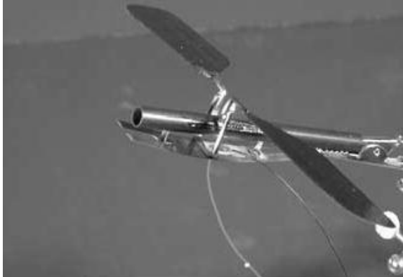
Figure 10: Unimorph actuated independently controlled wings [14]
