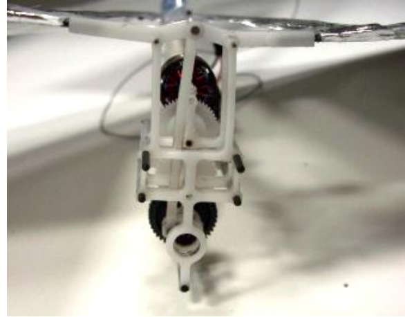
Figure 22: UMD single crank mechanism
