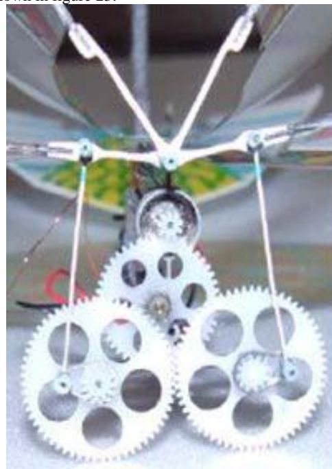
Figure 23: Parallel single cranks [24]
