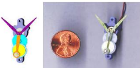
Figure 18: Double pushrod from Microbat [6]
