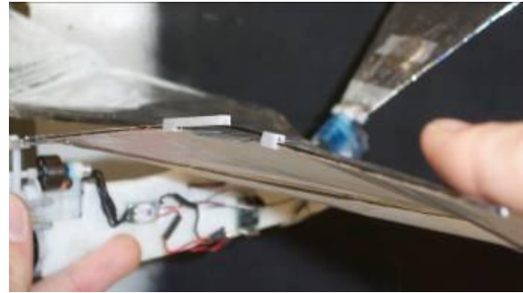
Figure 16: Wings with one-way compliance
