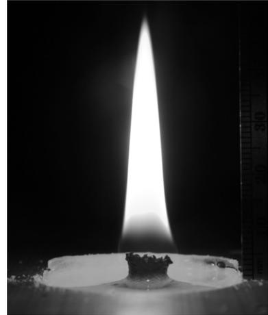
Fig. 3. Photograph of typical thick wick flame,  $D = 7.66$  mm.
