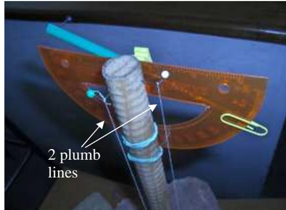
The purpose of the clinometer is to measure the angle  $a$  in the figure below. You can think of  $a$  as the angle between an imaginary horizontal line and the line-of-sight to the point "X".
