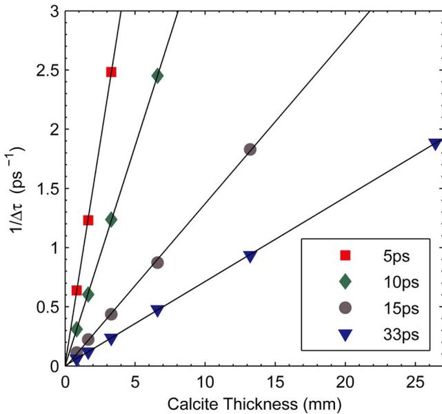
Fig. 3. (Color online) Plot of  $1/\Delta\tau$  as a function of the thickness of the multiple-order calcite wave plate for stretched pulses of duration 5, 10, 15, and 33 ps.
