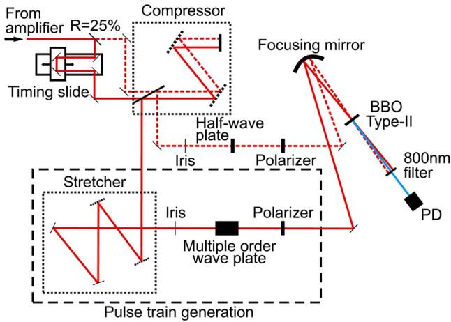
Fig. 1. (Color online) Experimental arrangement used to generate and measure trains of femtosecond pulses. PD, photodiode.
