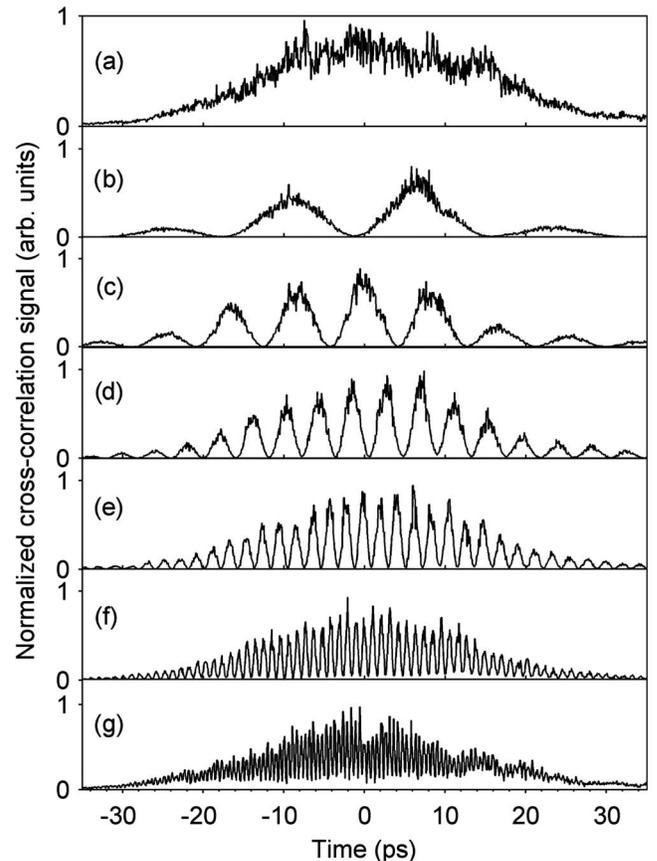
Fig. 2. Cross-correlation traces obtained with a stretched pulse of 33 ps FWHM duration and multiple-order calcite wave plates of thickness: (a) 0 mm (no crystal), (b) 0.83 mm, (c) 1.65 mm, (d) 3.30 mm, (e) 6.61 mm, (f) 13.22 mm, (g) 26.43 mm.
