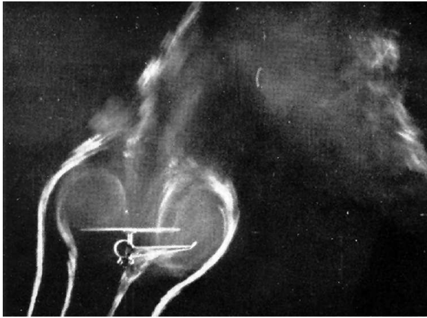
Figure 1: Smoke flow visualization of a rotor operating in the VRS, showing the characteristic recirculation of the flow in the rotor plane.
