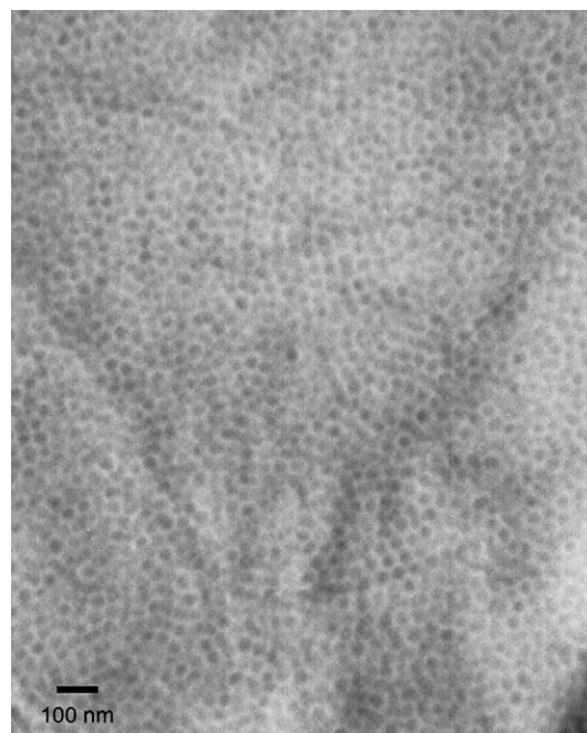
Fig. 7. PS/P4VP microtomed along the constraint direction, showing the cylinder ends. Contrast comes from nickel confined in the P4VP block.
