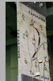
The bolted bonded composite experiment. Notice strain gauges and displacement flex bar.
